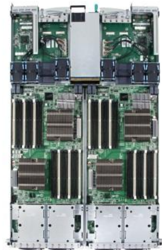
(Inside Top View of the SR-1600 1U Server Rack)
