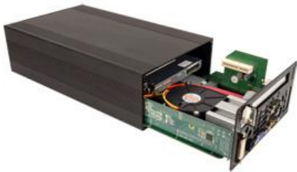
Rear/Inside PCI-e slot View
