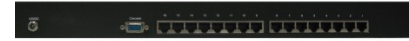
Close up of the Rear View of Cat-6 KVM showing Qty 16 RJ45 interface Ports
