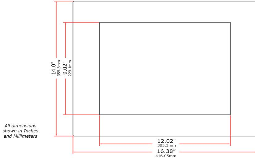
Note: max depth = 2.95" (74.93mm) with rear-mounted (removable) AC Adapter
