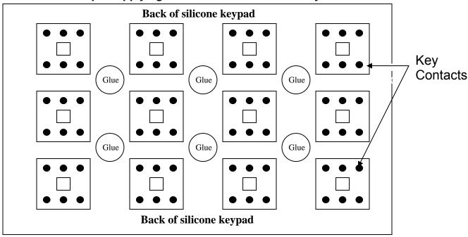
Apply silicone adhesive [Ùc^æc@recommends SuperFlex by Loctite] to back side of silicone overlay (keypad). Sparingly dab glue on the middle of each key intersection across the whole keyboard as seen in this picture. Also apply to inside of center portion of HulaPoint™ pad (where the sensor/joystick lies) if OEM kit incorporates the HulaPoint™
