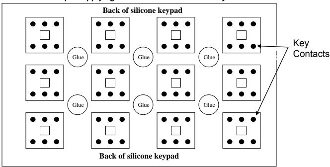
Apply silicone adhesive [Stealth recommends SuperFlex by Loctite] to back side of silicone overlay (keypad). Sparingly dab glue on the middle of each key intersection across the whole keyboard as seen in this picture.
